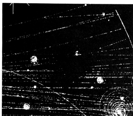
Pictures at left are from a photograph, made at Fermi National Accelerator Laboratory, of a high-energy proton producing 26 charged particles as a result of a collision with another proton. Courtesy Professor Gerald A. Smith, Michigan State University.
